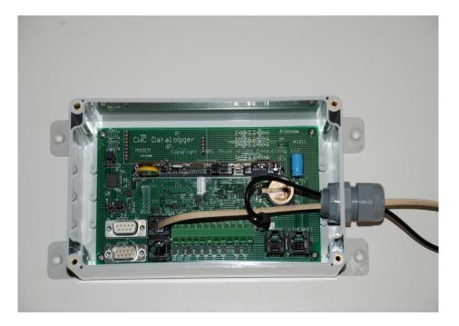
Now run the Ethernet cable (or phone line), plug it into the "Ethernet" (or "Phone") socket. Beware that the 1-wire connections use the same kind of modular connector as a phone. Do not mix them up!:
