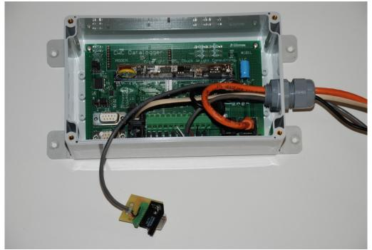
And plug in to the appropriate DB9 connector:
