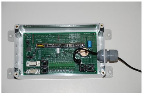
Next, run the 1-wire bus connection(s), if any. Either or both of the 1-wire sockets can be used. Discovery of 1-wire devices is automatic, and not dependent on which 1-wire port is used:
